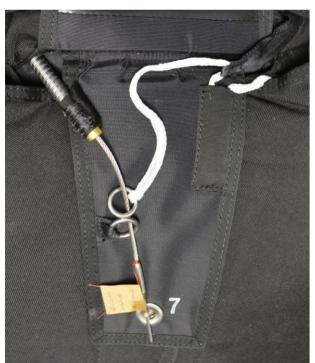
Figure no. 10 Notice: The cable of the reserve parachute ripcord including the needle must pass through the AOZP-RAX cord ring with 15 mm diameter and a spacer ring! Unused on purpose
