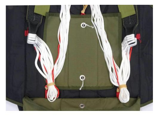
The lower part of the canopy with the placed lines is bent crosswise with the container and attached to the lower flap edge (pic. 24).
