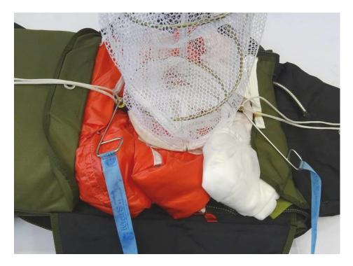
The auxiliary packing cords are passed through the tapes with metal grommets in the top part of the pilot chute, the pilot chute springs are pressed, the fabric of the canopy is placed in the centre direction between the spring threads, and the closing cord lugs are pulled out by means of auxiliary packing cords; the closing cord lugs are then secured with auxiliary packing mandrels (pic. 37).
