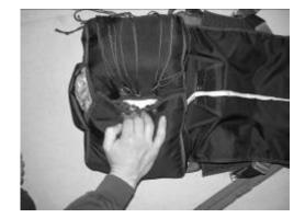
Now, we close the remaining half of the container. Remove one temporary pin and pull the pull-up so that the temporary locking loop appears. Secure the loop with a temporary pin. Repeat the same with the other temporary locking loop.
