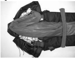
Now, we prepare one container side for closing. Cover the riser with the side closing flap and secure the flap by tucking the flap tab with velcro tape into the slit in the bottom of the container (also with velcro) (Fig. 37). Fig. 38 depicts the resulting shape of the container side.
