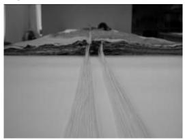
After pleating the canopy, check the suspension lines. Lift the upper risers with your right hand and separate the inner lines no.1 and 24 with the left hand (Fig.7). Slide your hands along the lines to the bottom of the canopy. There must be two distinct vertical halves (upper and lower) on the pleated canopy and the inner lines in your left hand must be lines marked no.1 and no. 24.
