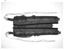
Cover the risers with the side flaps (Fig.19). Apply tension to the flaps and straighten the risers (Fig.20).
