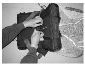
Once the closing cord is secured, cut the temporary tie (Fig. 65).
