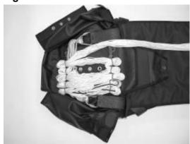
Continue packing (Fig. 31). The last line stow should be oriented as in Fig. 31. Place the canopy with the secured diaper in the left side of the container (Fig. 32).
