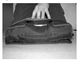
Use both knees to press the pilot chute against the container. Pull the closing cord and secure the pilot chute in the fully compressed position (Fig. 74).
