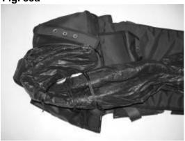
Make sufficient room for the pull-up cord and temporary locking loops around the grommets in the bottom of the container (Fig. 40). Pass the pull-up as well as the temporary locking loops through the grommets in the upper flap of the container and using the pull-ups and temporary pins (Fig. 41) secure the half of the container (Fig. 42).
