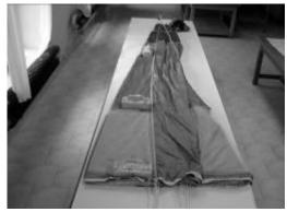
Straighten the canopy along its whole length and inspect the suspension lines. Straighten the lines and inspect them thoroughly from to skirt of the canopy to the SL-01 link connectors. Inspect the lines from all sides
