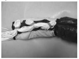
Move the harness together with the container and back padding towards the canopy (Fig 17). Route the risers as in Fig.18.
